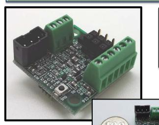
The sensor digital amplifier, C-sdAMP, has various advantages over conventional analog amplifiers: small, lightweight, low power, high precision, short lead-time for delivery, easy adjustment with PC connection, and less affected by temperature.
