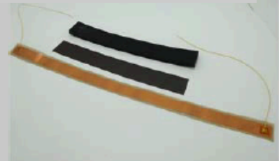
Power Receiving Coil (Three layers around the shaft)
